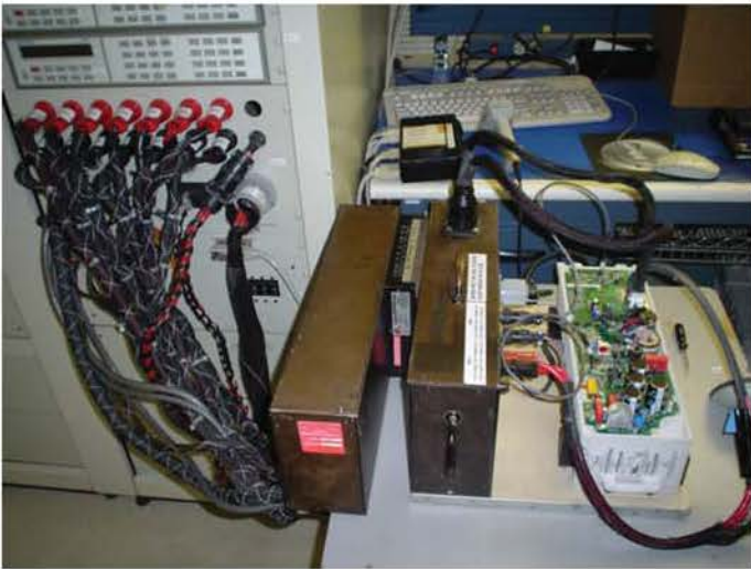
Close-Up view of Quick Connect to Production Interface Adapter with a Test Fixture and UUT
