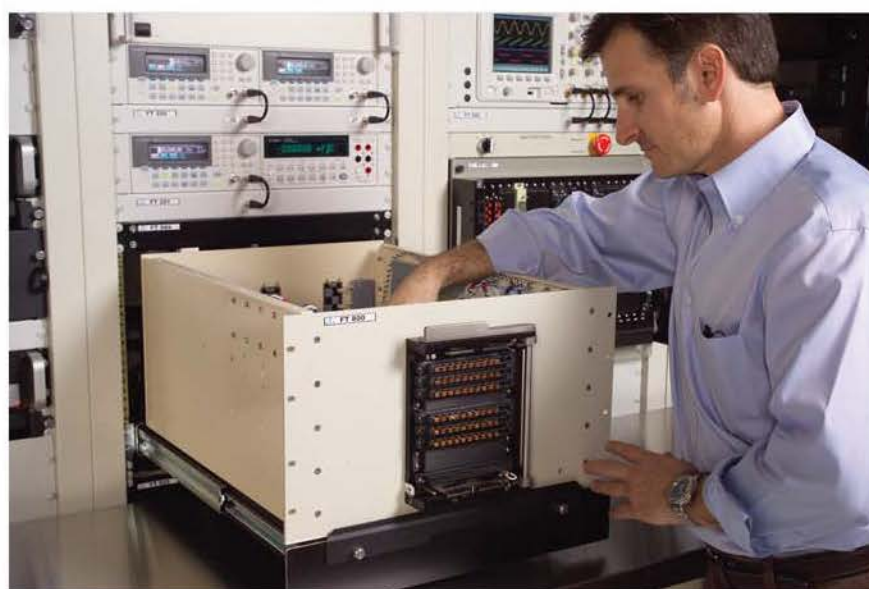
Front view close-up of DC Interface on pullout shelf showing easy access
