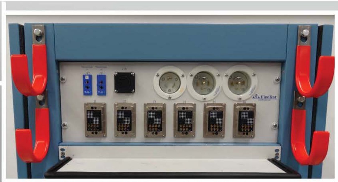
Rear System Interface Panel Close-Up showing Thermocouple Connections, AC Input Power Connections, 6 Unit Connections for Test Cables from Chamber to System, Cable Hooks for Test Cables
