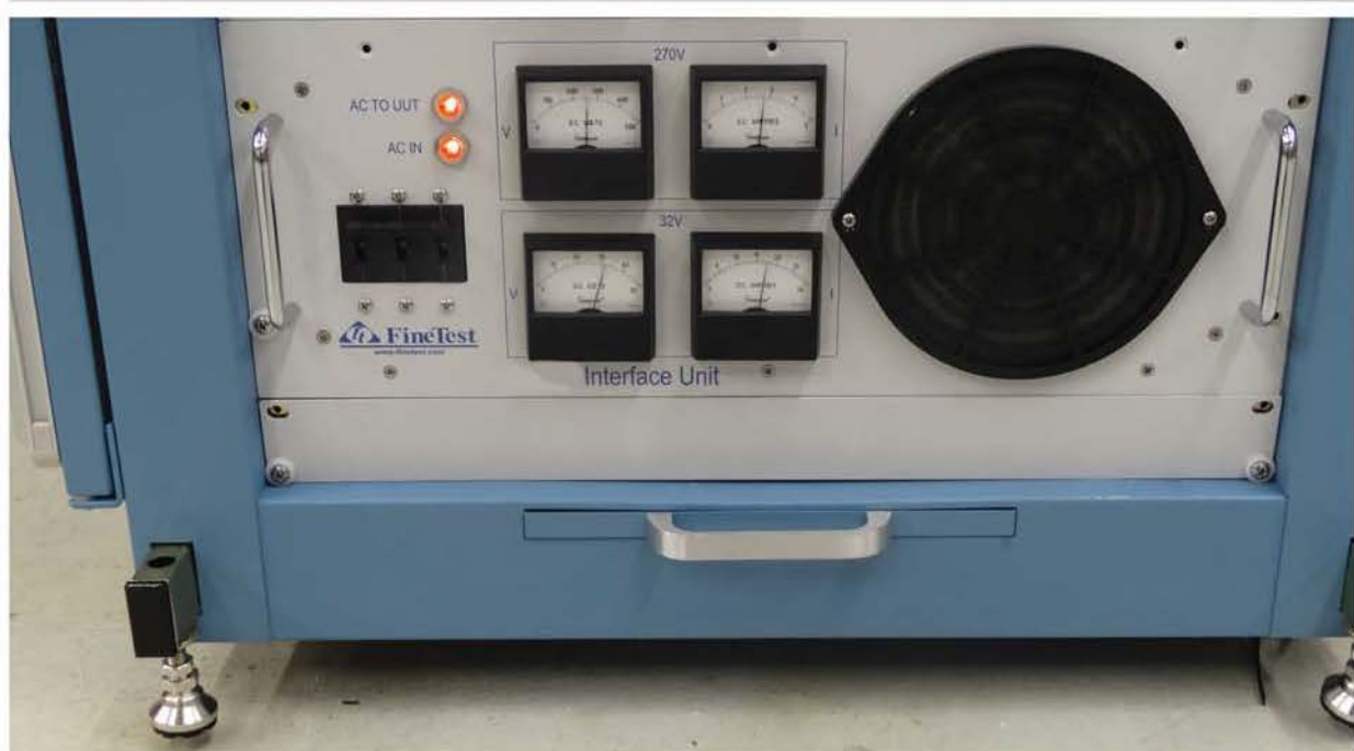
ESS UUT Interface Unit with Dual Voltage and Current Monitors and individually controlled AC Input On/Off with Circuit Breaker and Indicators
