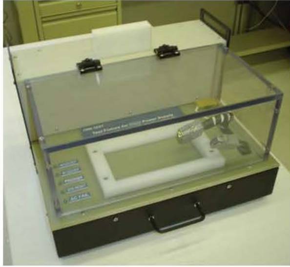
Front view of an ITA showing UUT Status Line LEDs
