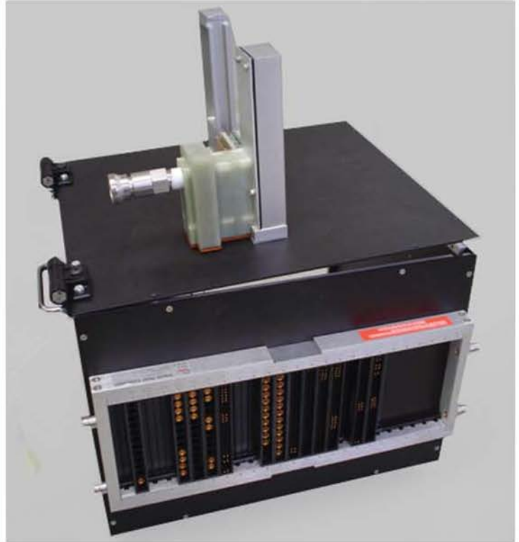
ITA with hookup for Thermal Hood on top where the UUT is plugged in
