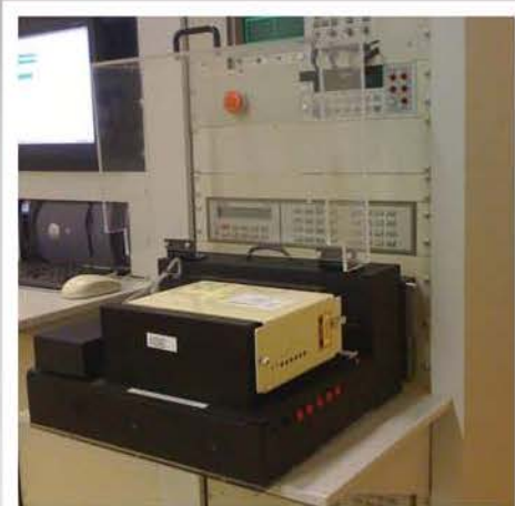
Close-Up Test Fixture with UUT
