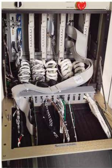
Close-Up ARINC Interface dropped down showing VXI Chassis and Cards (All signals routed through Ferrite Cores)
