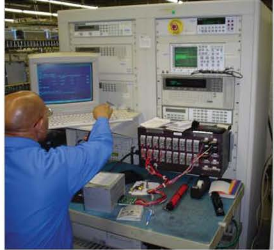
Operator testing a UUT
