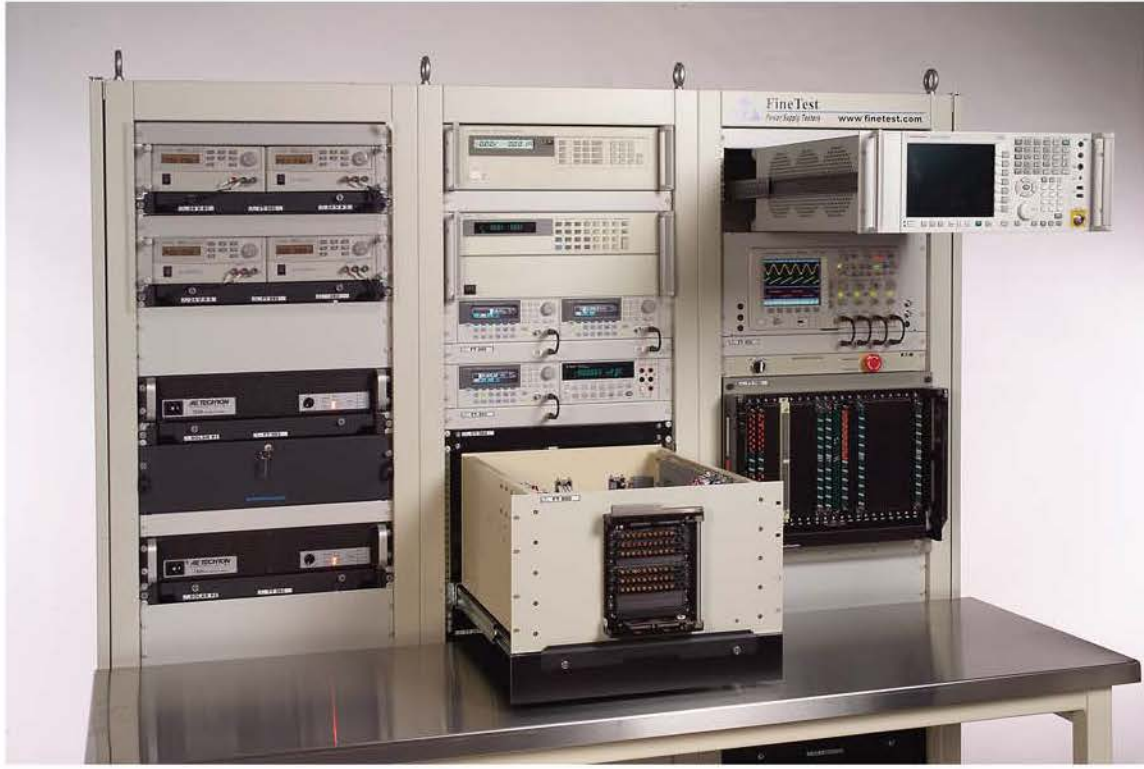
Front view of Tester showing all equipment on pull out shelves
