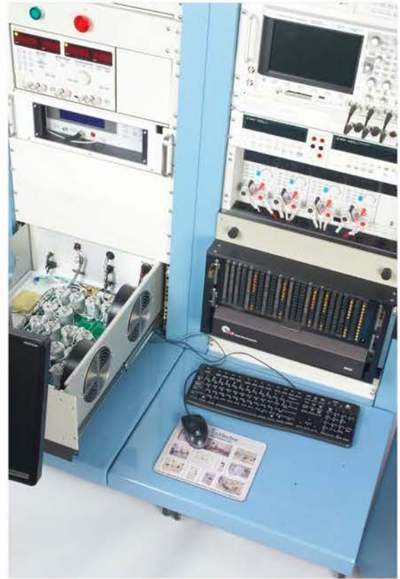
Front top view of Tester showing DC Interface box with sliding rails
