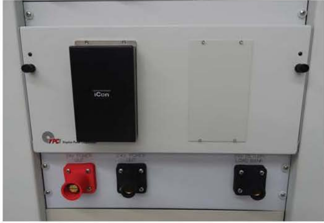
Front Panel Interface with VPC and High Power
